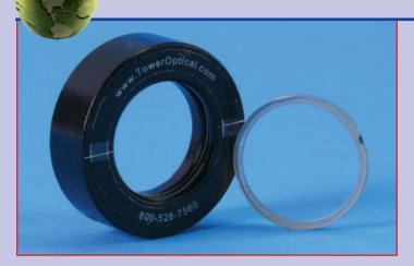
**Tower's 17.5 mm HLD zero order waveplates** provide users with a high performance crystal quartz retarder with a clear aperture of 15 mm. These waveplates are air spaced, having a stainless steel spacer betweentwo crystal quartz plates that form the zero order capability.
